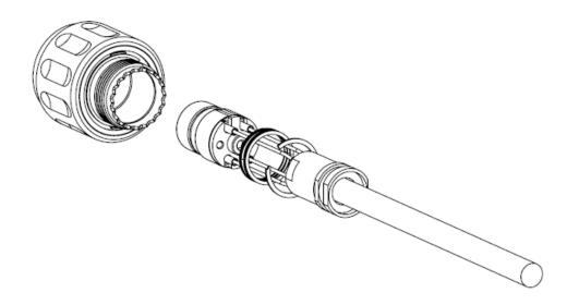
Slide the Wave Spring up behind the Insert. Install the Snap Ring behind the Wave Spring into the Snap Ring groove to hold Insert in place.
