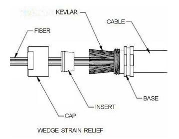
Screw on Wedge Strain Relief Cap to the Wedge Strain Relief Base. Tighten using the Dial Torque-Measuring Wrench PT-506 and Crow's Foot Wrench PT-536 and torque to the values in the above Torque Table.
