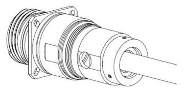
Pull Strain Relief to bottom of Backshell Retainer and tighten set screws using Hex Driver PT-500. Use Torque Hex Driver PT-590 with Hex Bit 0.050" PT-599 and torque Set Screws to the values in the above Torque Table. Perform a final visual check by looking through the holes in the Backshell Retainer to make sure that the fiber is not twisted or kinked.
