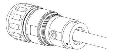
Pull Strain Relief to bottom of Spacer and tighten Set Screws using Hex Driver PT-500. Use Torque Hex Driver PT-590 with Hex Bit 0.050" PT-599 and torque Set Screws to the values in the above Torque Table. Perform a final visual check by looking through the holes in the Spacer to make sure that the fiber is not twisted or kinked.
