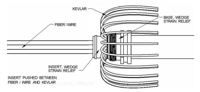
Cut Kevlar flush with top of wedge. Screw on Cap of Wedge Strain Relief. Torque to tighten using values from Torque Table above.
