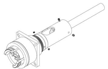
VC-3 Threadmate on the threads per manufacturer's instructions. Then use Torque Hex Driver PT-590 with Hex Bit .050" PT-599 and torque to the values in the above Torque Table.
