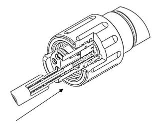
**For MT Insert** – Use MT Termini Insertion / Removal Tool PT-480 and slip Spring Push onto the prongs on the "insert" side of the tool and push MT Ferrule into the back cavity of the MT Insert. MT Ferrule should snap into place.
