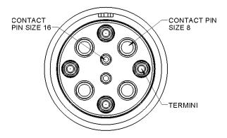
When populating using APC Fiber Optic Termini, align the key on the Fiber Optic Termini with keyway in the Insert.
